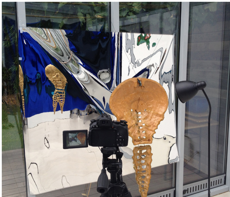
Fig. 8. Assembly used for obtaining images of sculptures in distorted mirror foil.
